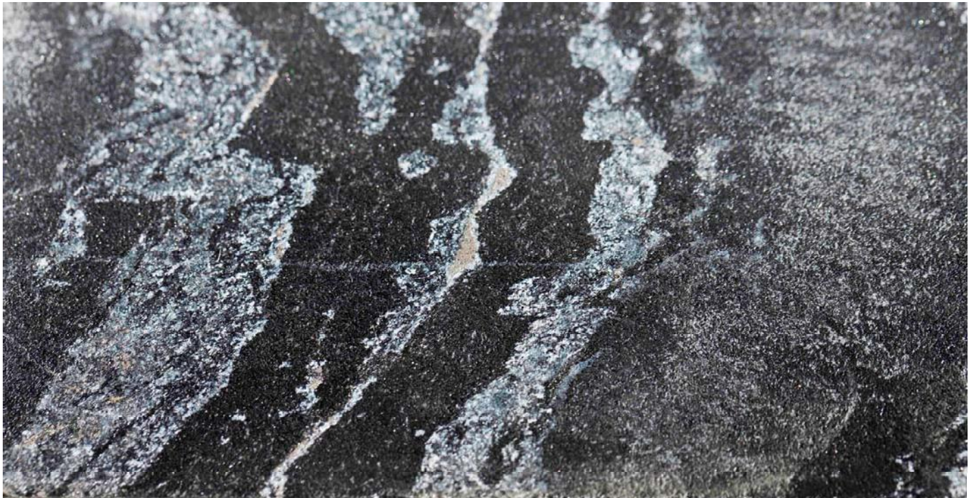
Core photo of KRD10-02 – 128.5 metres : banded biotite-quartz-carbonate schist with disseminated pyrite and uraninite. (50mm from top to bottom)
