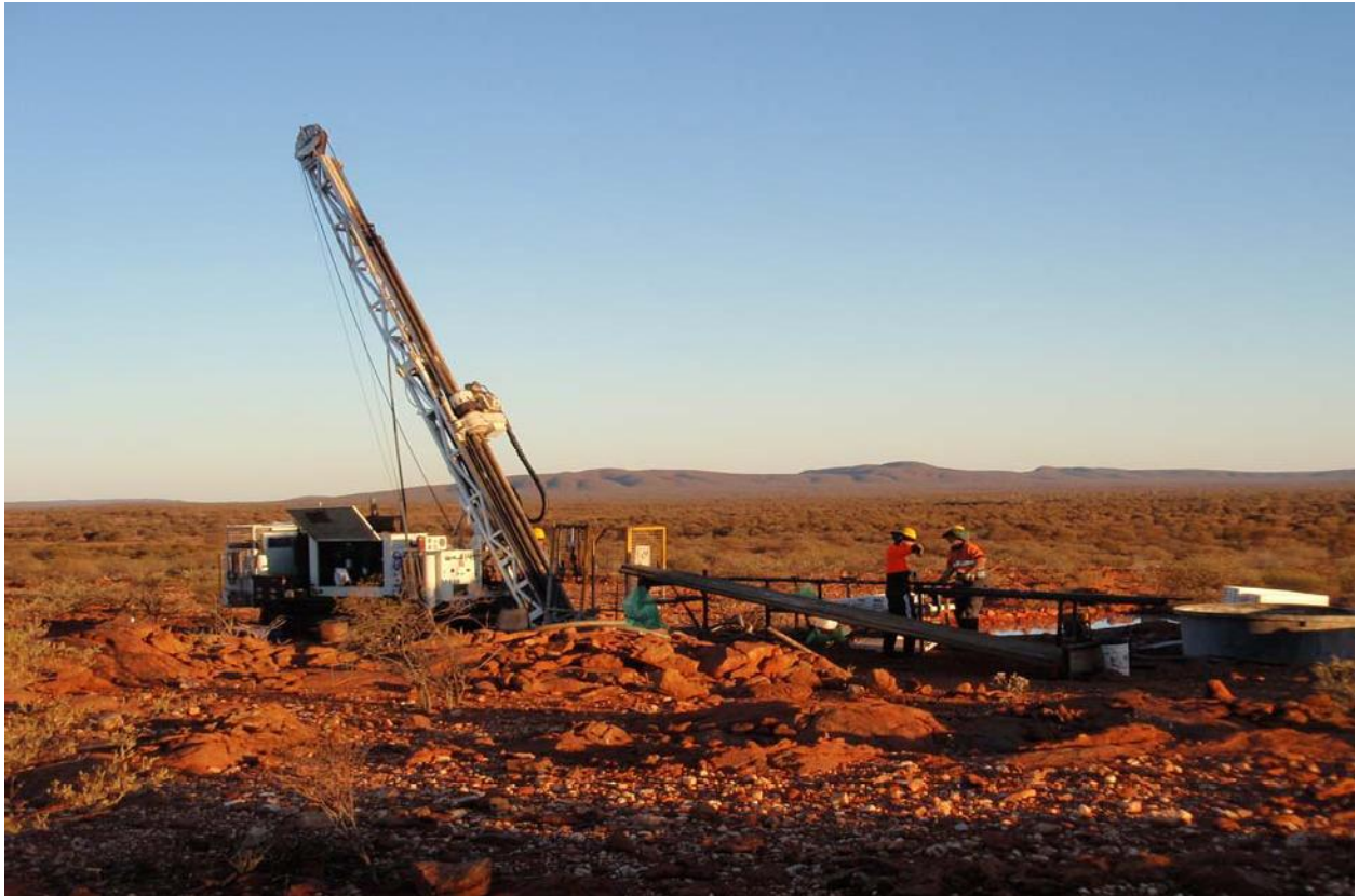
Diamond core drilling at Yarlarweelor's Doris uranium prospect – WA
